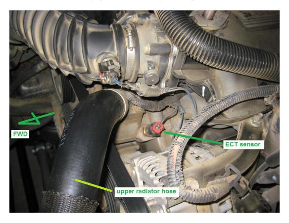
If the hose collapses or you hear bubbles then you have air in the system. This may be a minor problem or it could be a symptom of something more serious. (Possible causes include empty recovery tank, bad radiator cap, or even blown head gasket.)
