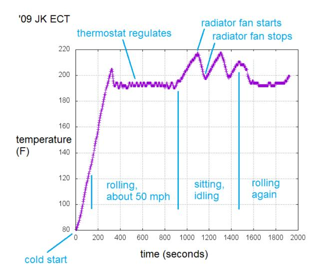
Before the engine reaches normal operating temperature (about 195 F) the thermostat is closed.
