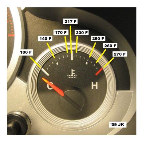
On the left side the small divisions are about 10 F each. Then there are about 50 degrees crammed into the one division on the left side of center scale. This is apparently by design. I suppose they didn't want the customer to see the 20 F swings when the fan runs.
