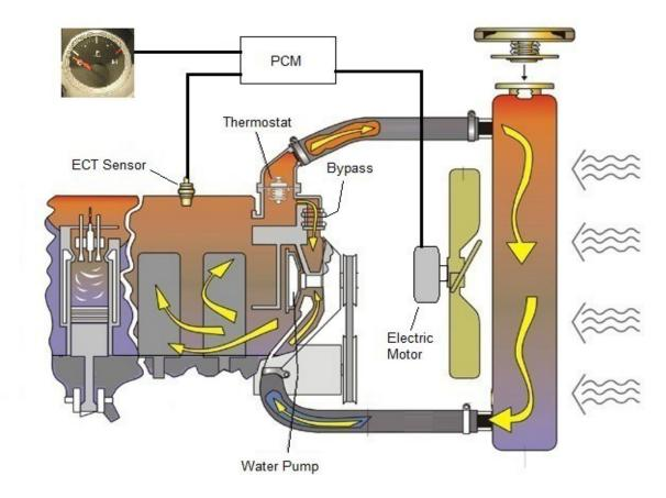
Combustion is affected by cylinder and head temperature. The cooling system tries to control the temperature at a relatively fixed optimum temperature. Then the spark timing and mixture are adjusted for optimum combustion depending on load, air density, etc.
